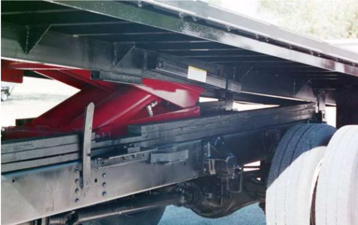
This is a model D-22-H Dewey Hoist in a 15 Ton installation showing prop.
